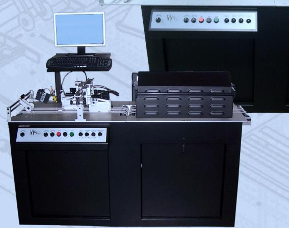
Our split base transports utilize independent transport belts engineered specifically for your inkjet and drying applications requiring IR, NIR and UV drying and inkjet technologies and are available in a variety of belt configurations as well single and dual motor drive versions.
